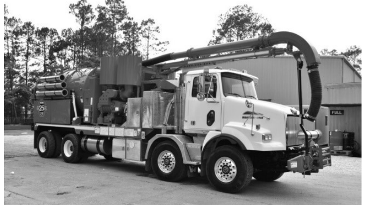
Typical JetVac Truck
