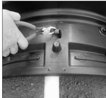
9. Remove tongue of connector hook.
