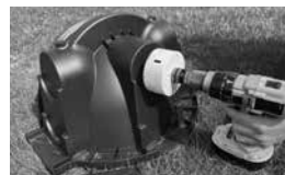
2. Drill the hole on the endcap.
