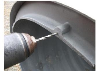
Figure 6: Chucked Vent Plug
