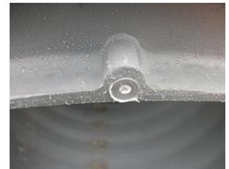
11. If necessary, the welded area can be cleaned up with a sureform tool or similar scraping device (see Figure 10).
