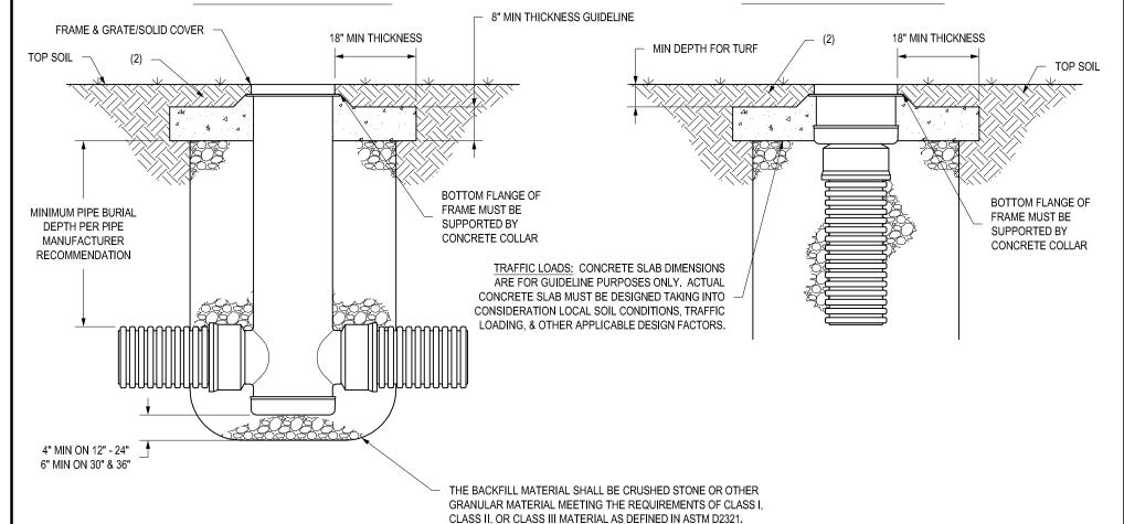
BEDDING & BACKFILL FOR SURFACE DRAINAGE INLETS SHALL BE PLACED & COMPACTED UNIFORMLY IN ACCORDANCE WITH ASTM D2321.
