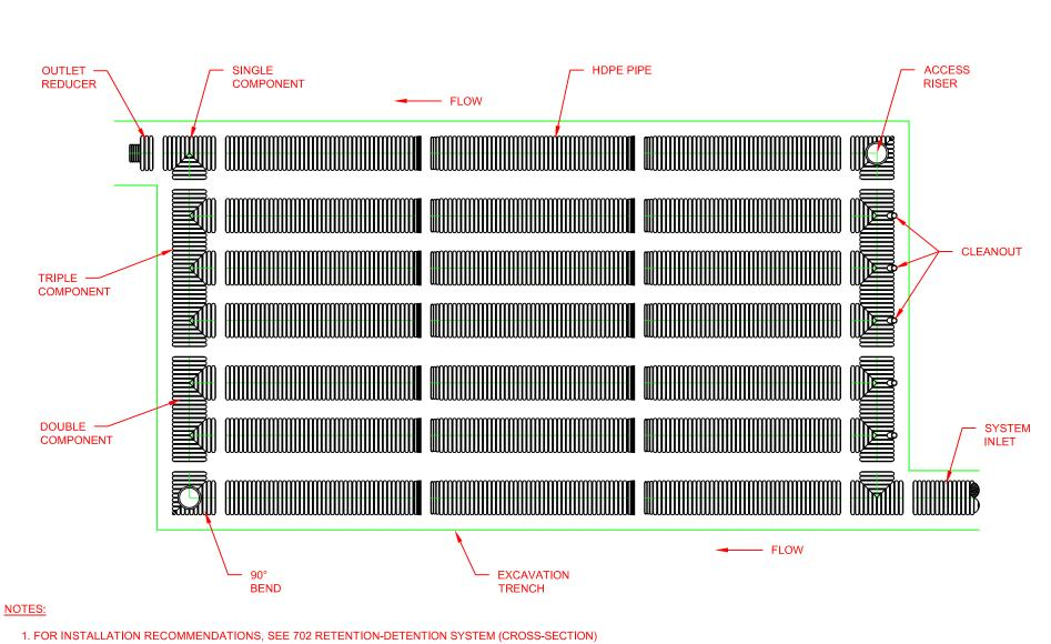
AND 703 RETENTION-DETENTION SYSTEM (RISER AND CLEANOUTS)
