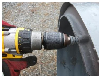
Figure 8: Holding Drill Flush
