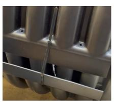
5. Repeat step four on the other side of the pipe, threading the zip tie through the outside of the coupler and continue working it through the hole on the inside of the part.
