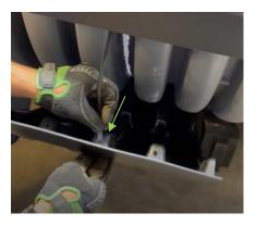
c. Continue to feed the zip tie through until the two halves of the coupler can be brought together and the zip tie can be cinched together.
