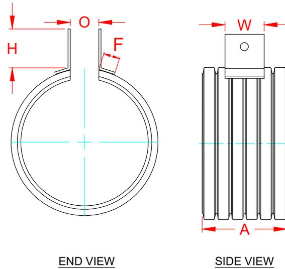
**SHEET STOCK COUPLER FOR 12 IN - 36 IN PIPE DIAMETER**
