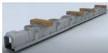
2x4's (0.6x1.2 m) can be fastened to provide a wider footing.
