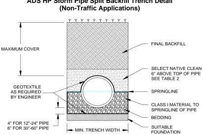
Figure 1 ADS HP Storm Pipe Split Backfill Trench Detail (Non-Traffic Applications)
