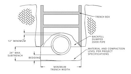
In installations not involving a subtrench, dragging a trench box should only be done if it does not damage the pipe or disrupt the backfill; otherwise, the box should be lifted vertically into its new position, again taking great care not to disturb the pipe or backfill.
