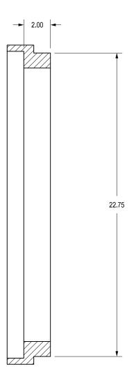
QUALITY: MATERIALS SHALL CONFORM TO ASTM A536 GRADE 70-50-05 PAINT: CASTINGS ARE FURNISHED WITH A BLACK PAINT DIMENSIONS ARE FOR REFERENCE ONLY
