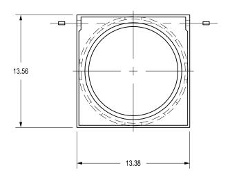
DIMENSIONS ARE FOR REFERENCE ONLY ACTUAL DIMENSIONS MAY VARY DIMENSIONS ARE IN INCHES GRATE MEETS H-20 LOAD RATING QUALITY: MATERIALS SHALL CONFORM TO ASTM A536 GRADE 70-50-05 PAINT: CASTINGS ARE FURNISHED WITH A BLACK PAINT LOCKING DEVICE AVAILABLE UPON REQUEST SEE DRAWING NO. 7001-110-033
