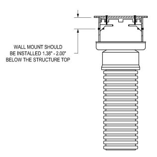
LOCKING DEVICE SHALL BE STAINLESS STEEL TO BE USED WITH PVC RISER ONLY
