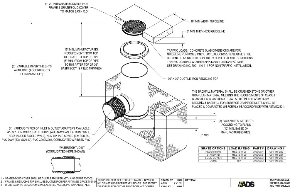
3 - DRAIN BASIN TO BE CUSTOM MANUFACTURED ACCORDING TO PLAN DETAILS. RISERS ARE NEEDED FOR BASIN BODIES OVER 84" DUE TO SHIPPING RESTRICTIONS.
