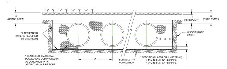
MINIMUM H (GRASS) = 12" FOR 12" THROUGH 60" HDPE PIPE MINIMUM H (FLEX PVMT), H (RIGID PVMT) = 12" FOR UP TO AND INCLUDING 36" HDPE PIPE = 24" FOR 42" THROUGH 60" HDPE PIPE
