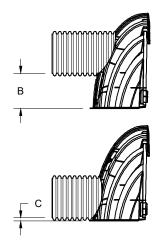
**CUSTOM PREFABRICATED INVERTS** ARE AVAILABLE UPON REQUEST. INVENTORIED MANIFOLDS INCLUDE 300-600 mm (12-24") SIZE ON SIZE AND 375-1200 mm (15-48") ECCENTRIC MANIFOLDS. CUSTOM INVERT LOCATIONS ON THE MC-4500 END CAP CUT IN THE FIELD ARE NOT RECOMMENDED FOR PIPE SIZES GREATER THAN 250 mm (10"). THE INVERT LOCATION IN COLUMN 'B' ARE THE HIGHEST POSSIBLE FOR THE PIPE SIZE.
