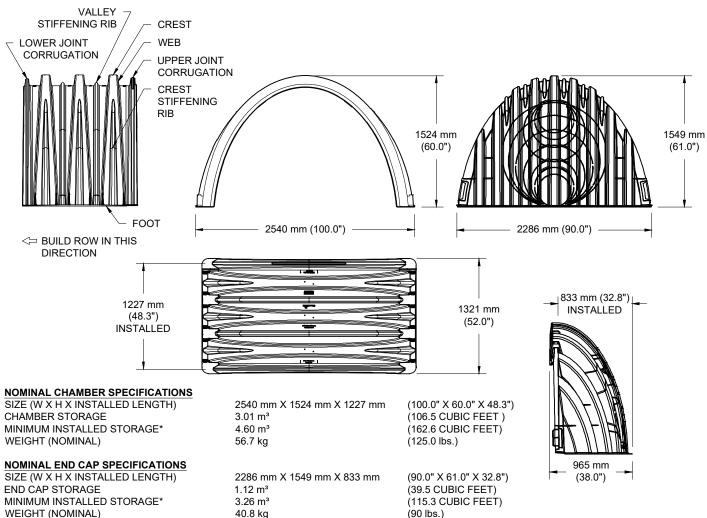
\*ASSUMES 305 mm (12") STONE ABOVE, 229 mm (9") STONE FOUNDATION AND BETWEEN CHAMBERS, 305 mm (12") STONE PERIMETER IN FRONT OF END CAPS AND 40% STONE POROSITY.
