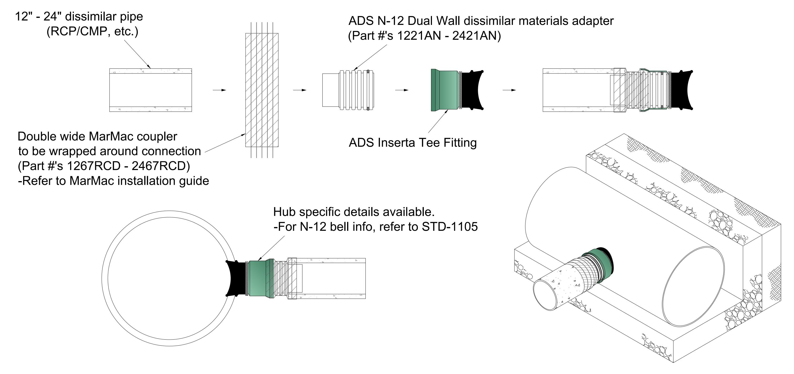
NOTE: FOR DISSIMILAR NEEDS SMALLER THAN 12", USE INSERTA TEE FITTINGS FOR SDR35 PVC OR SCH40 PVC (PER STD-1106, STD-1109, OR STD-1108) AND A COUPLER OR ADAPTER (BY OTHERS) TO ACHIEVE CONNECTION.
