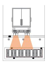
For vehicle loading, an additional impact factor is used to ensure adequate cover. The impact factor is calculated based upon the height of fill between the surface and the top of the ACQUABOX system. For minimum cover installations, the load is increased by up to 33% and will reduce as fill height increases.
