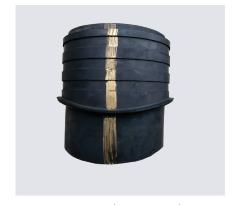
Assemble the two sleeves together so that about 2"-3" (50-75 mm) of the inner sleeve is visible. The inner sleeve should not protrude through the wall of the host pipe. Be sure the gold line on each sleeve is aligned.
