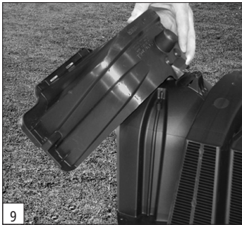
Attach endcap to last chamber.
