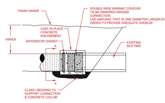
**CAST IN PLACE** CONCRETE DOUBLE WIDE MARMAC **ENCASEMENT** COUPLER TO BE WRAPPED AROUND CONNECTION
