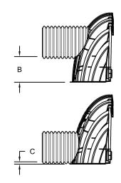
CUSTOM PREFABRICATED INVERTS ARE AVAILABLE UPON REQUEST. INVENTORIED MANIFOLDS INCLUDE 12-24" (300-600 mm) SIZE ON SIZE AND 15-48" (375-1200 mm) ECCENTRIC MANIFOLDS. CUSTOM INVERT LOCATIONS ON THE MC-7200 END CAP CUT IN THE FIELD ARE NOT RECOMMENDED FOR PIPE SIZES GREATER THAN 10" (250 mm). THE INVERT LOCATION IN COLUMN 'B' ARE THE HIGHEST POSSIBLE FOR THE PIPE SIZE.
