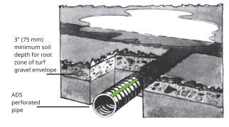
Use perforated pipe, installed in gravel, to collect and carry water to catch basin/ disposal area. In heavy clay soils, several lines of perforated pipe may be needed to speed drainage.
