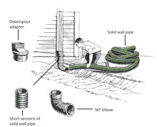
To carry rainwater away from the house and avoid water seeping down basement walls and creating wet basement problems, use solid wall pipe from downspout to storm drain inlet, street curb or other disposal area.
