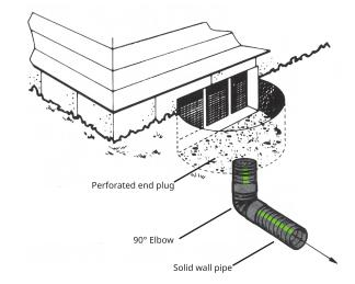
Basement window wells should be drained to prevent water from seeping down to the foundation wall and entering the basement.
