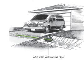
To carry water beneath your driveway, use solid wall pipe. Crushed stone, gravel or compacted soil backfill material should be used as the bedding material around the culvert, with aggregate size not exceeding 1" (25 mm). Minimum recommended cover is 12" (300 mm). For driveway culverts with less than 12" (300 mm) of cover see ADS Pocket Installation Guide.
