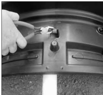
9. Remove tongue of connector hook.
