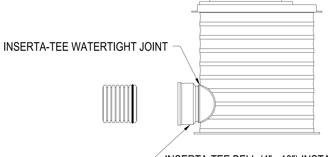
INSERTA-TEE BELL (4" - 10") INSTALLED DURING FABRICATION INSERTA-TEE FITTING CAN ALSO BE INSTALLED IN FIELD OTHER PIPE CONNECTIONS AVAILABLE (NOT SHOWN, INQUIRE)
