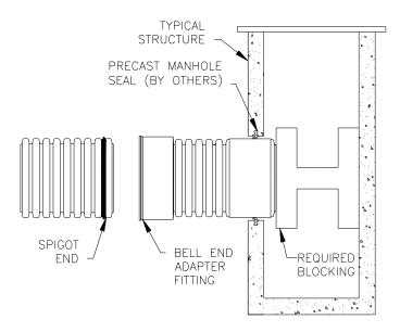
Alternately, when using the adapter fitting in the downstream end of the structure, before pushing the bell and spigot together from inside the structure, it is necessary to provide blocking at the structure to prevent the fitting from moving in the structure, as shown to the left.
