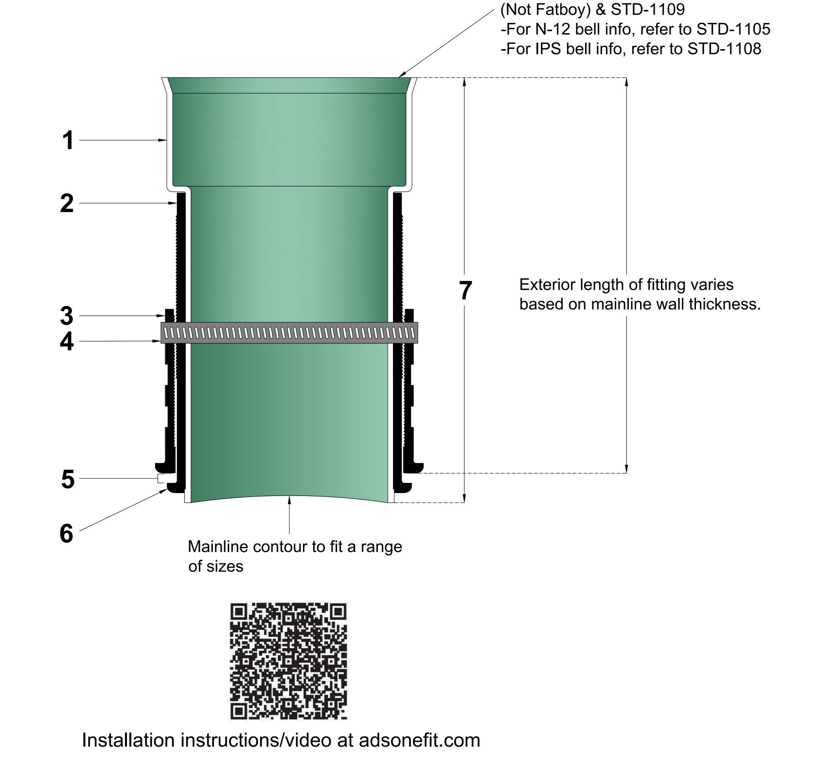
NOTE: FOR INSTALLATION INSTRUCTIONS, REFER TO DETAIL STD-1100. FOR PROTRUSION INFORMATION, REFER TO DETAIL STD-1101. FOR HOLE SAW INFORMATION, REFER TO DETAIL STD-1102.
