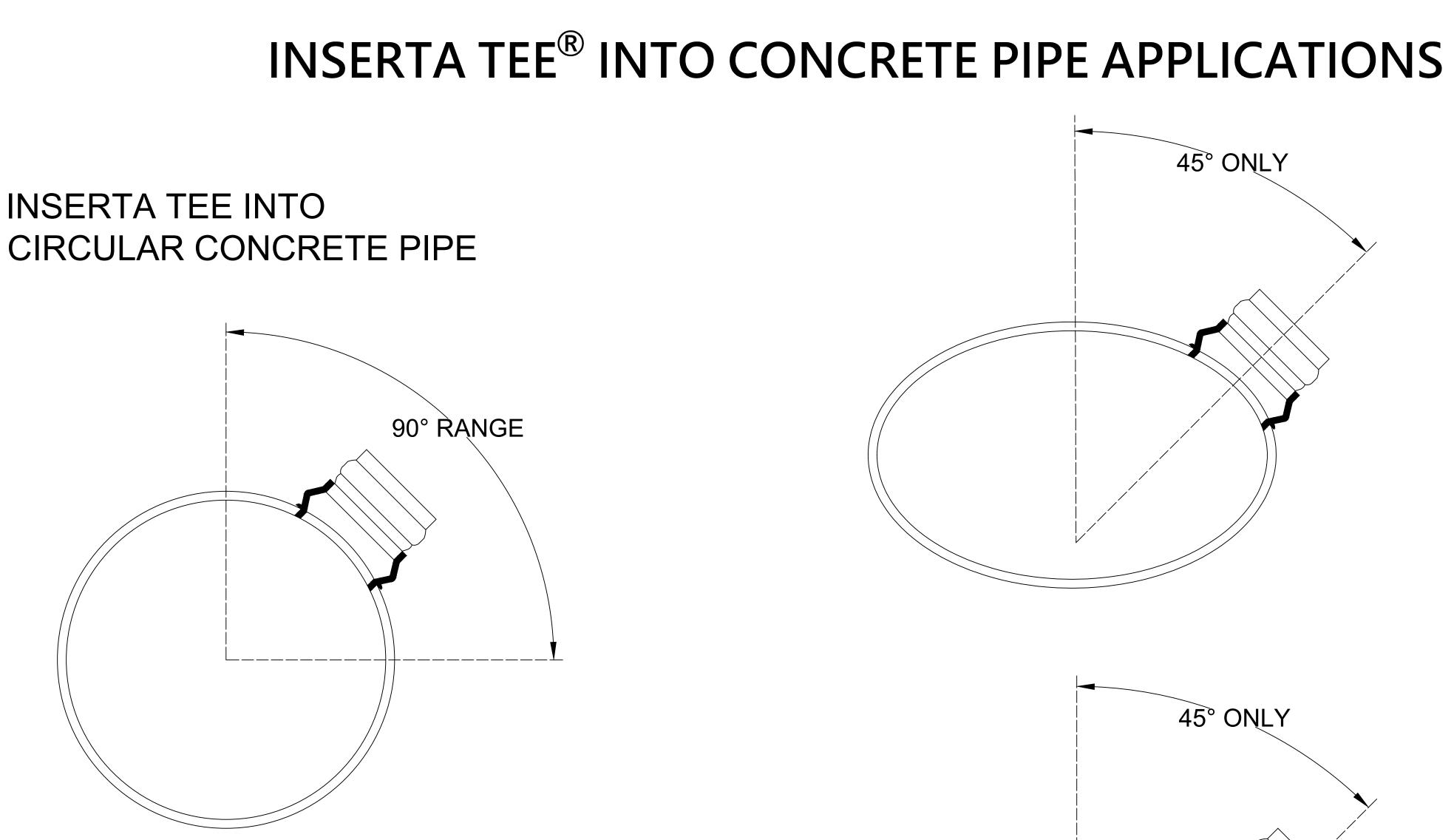
For circular pipe, installation angle of Inserta Tee can range anywhere between 0° and 90°, with typical installations at a 45° angle as seen in detail above.
