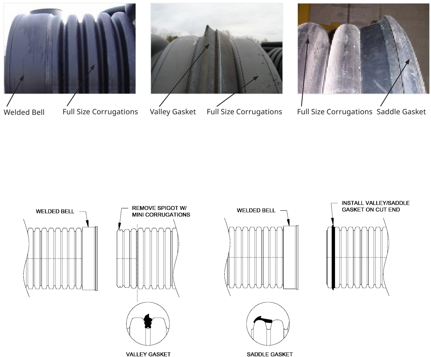
Figure 2: Welded Bell Connection
