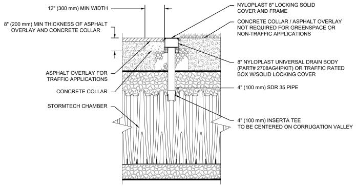
NOTE: INSPECTION PORTS MAY BE CONNECTED THROUGH ANY CHAMBER CORRUGATION VALLEY.
