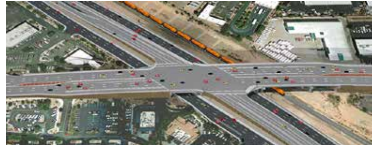
The new interchange is a median urban diamond design (see inset photo), with traffic now diverted over the railroad tracks.
