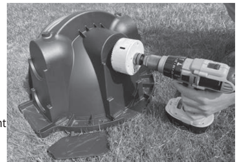
2. Drill the hole on the endcap.
