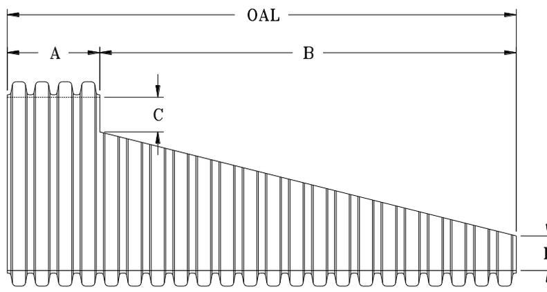
Note: ADS recommends that the product be installed with a concrete collar/edge to support and close corrugations per DOT specifications. The Channel at the bottom of the taper must be shaped to prevent toe lift by the inlet water flow.
