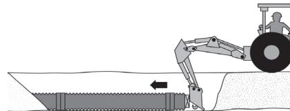
*NOTE: This method requires use of installation stub. DO NOT push backhoe directly against pipe.*
