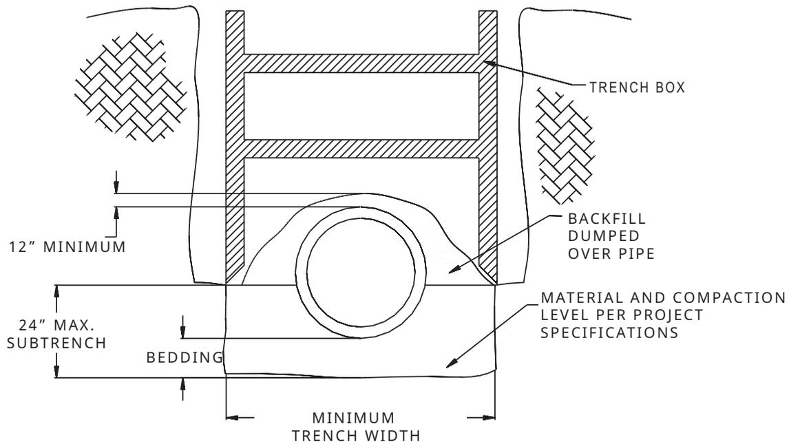
In installations not involving a subtrench, dragging a trench box should only be done if it does not damage the pipe or disrupt the backfill; otherwise, the box should be lifted vertically into its new position, again taking great care not to disturb the pipe or backfill.
