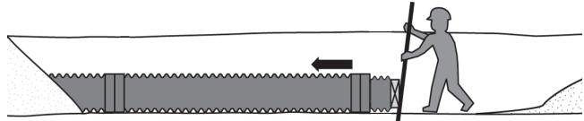
*NOTE: This method requires use of installation stub. DO NOT push directly against pipe.*
