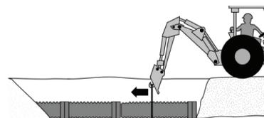
*NOTE: Distance from bedding to bottom of pipe not to exceed 6" (150 mm) for a 20' (6 m) pipe.*
