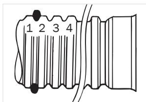
*Gasket printing should be visible in this location when properly installed.*
