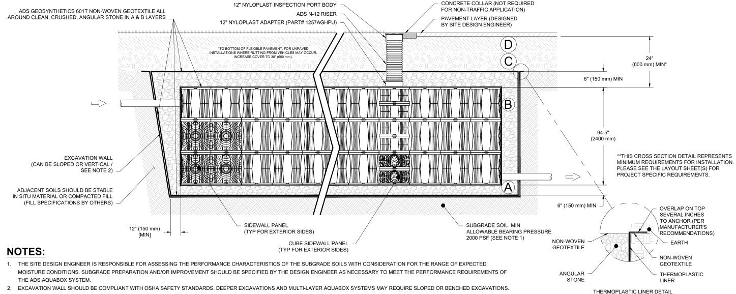
PERIMETER STONE MUST BE EXTENDED HORIZONTALLY TO THE EXCAVATION WALL
