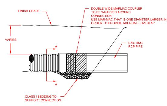
DOUBLE WIDE MARMAC **COUPLER TO BE** WRAPPED AROUND CONNECTION SECTION "A-A"
