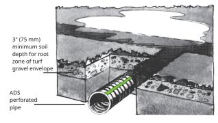
Use perforated pipe, installed in gravel, to collect and carry water to catch basin/ disposal area. In heavy clay soils, several lines of perforated pipe may be needed to speed
