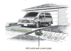
To carry water beneath your driveway, use solid wall pipe. Crushed stone, gravel or compacted soil backfill material should be used as the bedding material around the culvert, with aggregate size not exceeding 25 mm (1"). Minimum recommended cover is 300 mm (12"). For driveway culverts with less than 300 mm (12") of cover see ADS Pocket Installation Guide.
