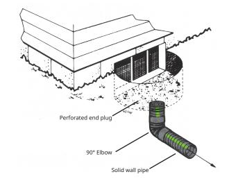
Basement window wells should be drained to prevent water from seeping down to the foundation wall and entering the basement.
