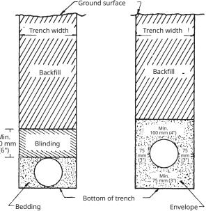
Pipe encased in bedding for support (left) and pipe encased in sand and gravel envelope designed as filter (right
