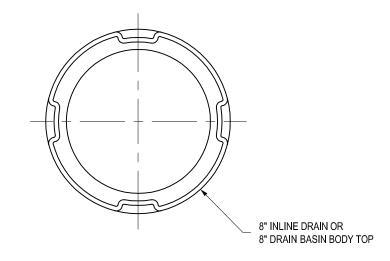
DIMENSIONS ARE FOR REFERENCE ONLY ACTUAL DIMENSIONS MAY VARY DIMENSIONS ARE IN INCHES GRATE HAS LIGHT DUTY RATING
