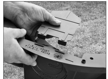
4. Install splash plate.
