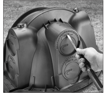
1. Start tear-out seal.
