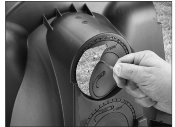
2. Pull tab on tear-out seal.
