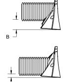
ALL STUBS, EXCEPT FOR THE SC310ECEZ ARE PLACED AT BOTTOM OF END CAP SUCH THAT THE OUTSIDE DIAMETER OF THE STUB IS FLUSH WITH THE BOTTOM OF THE END CAP. FOR ADDITIONAL INFORMATION CONTACT STORMTECH AT 1-888-892-2694.
