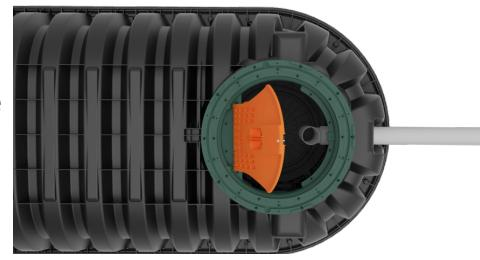
3. Reduce the torque and speed of your drill driver and screw the (10) #14 2" stainless steel screws into the screw bosses located on either the outer or inner ring of the adapter to complete the connection between the Guardian and EZsnap riser.
