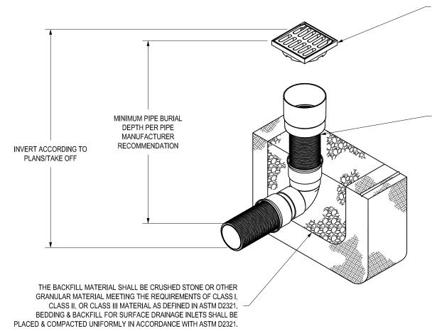
INTEGRATED DUCTILE IRON FRAME & GRATE TO MATCH UNIVERSAL INLINE DRAIN O.D.
