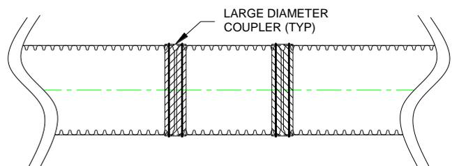
The couplers are used by removing the damaged section of pipe, replacing it with a new section and then sliding the coupler back around the joint, similar to the slip coupling above. The couplers stainless steel bands are then tightened to the manufactures recommendations. These rubber couplings are capable of meeting watertight field test requirements when installed per the manufacturer's recommendations.
