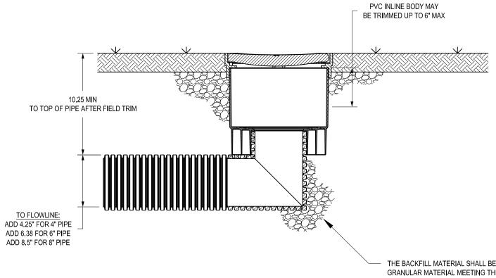
THE BACKFILL MATERIAL SHALL BE CRUSHED STONE OR OTHER GRANULAR MATERIAL MEETING THE REQUIREMENTS OF CLASS I, CLASS II, OR CLASS III MATERIAL AS DEFINED BY ASTM D2321. BEDDING & BACKFILL SHALL BE WELL PLACED AND COMPACTED UNIFORMLY IN ACCORDANCE WITH ASTM D2321.
