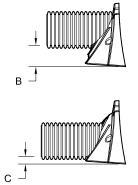
TOUS LES TUYAUX, SAUF POUR LE SC310ECEZ, SONT PLACÉS AU PIED DU BOUCHON DE SORTE QUE LE DIAMÈTRE EXTÉRIEUR DU TUYAU SOIT AU MÊME NIVEAU QUE LE PIED DU BOUCHON. POUR DE L'INFORMATION COMPLÉMENTAIRE CONTACTER ADS CANADA AU 819-395-4244.
