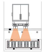
For vehicle loading, an additional impact factor is used to ensure adequate cover. The impact factor is calculated based upon the height of fill between the surface and the top of the Aquabox system. For minimum cover installations, the load is increased by up to 33% and will reduce as fill height increases.
