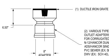
(2) VARIOUS TYPES OF INLET & **OUTLET ADAPTERS AVAILABLE:** FOR CORRUGATED HDPE (ADS N-12/HANCOR DUAL WALL, ADS/HANCOR SINGLE WALL), PVC SEWER (EX: SDR 35), PVC DWV (EX: SCH 40), PVC C900/C905, CORRUGATED & RIBBED PVC
