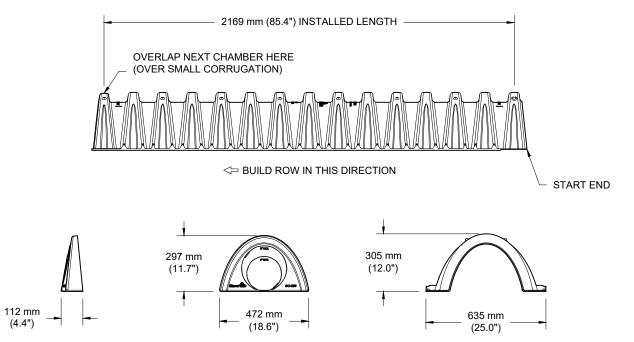
NOMINAL CHAMBER SPECIFICATIONS SIZE (W X H X INSTALLED LENGTH) CHAMBER STORAGE MINIMUM INSTALLED STORAGE\*
