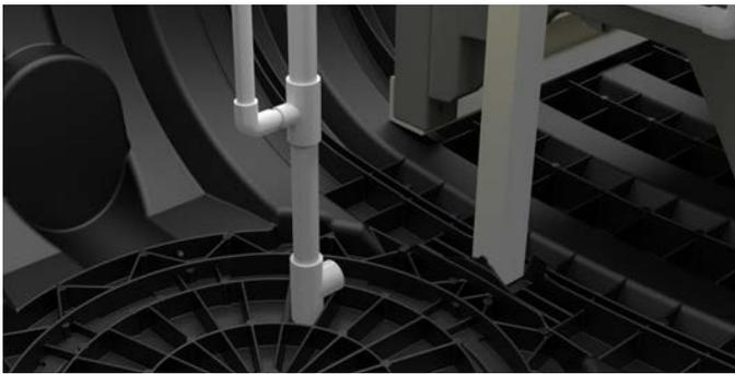
Attach the Reducer Assembly to the Air Grid Extension as shown below matching the ends labeled "B".
