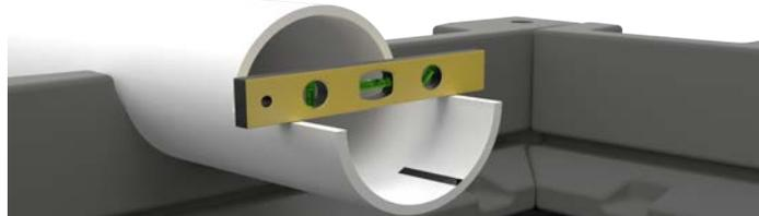
The reactor tank outlet tee assembly should be solvent welded to the outlet pipe and must extend six to twelve inches into the outlet side of the tank. The reactor tank inlet piping should be sloped downward toward the ECOPOD media and the outlet piping should sloped downward and away from the tank.
