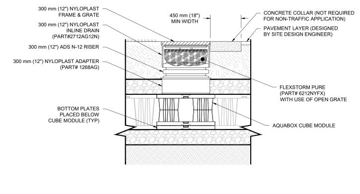
AQUABOX INSPECTION PORT INLET W/FLEXSTORM DETAIL NTS
